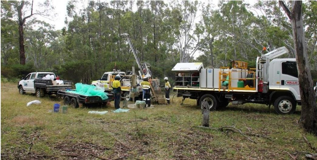
6. **Diamond Drilling** to extract a continuous cylindrical core of rock. The rig is usually truck mounted and generally requires two support trucks and at least one support light vehicle. Water is used to lubricate and cool the diamond-tipped drill equipment in the hole. Diamond drilling can deliver rock sample from over 1,000m below surface but is one of the most expensive and time consuming drilling techniques available. A single 250m diamond hole may take up to 5 days to drill (24 hour/day);
